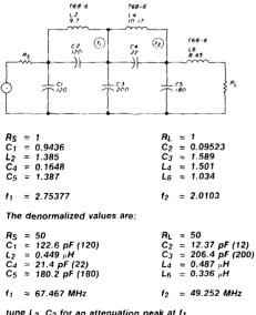
tune L<sub>2</sub>, C<sub>2</sub> for an attenuation peak at  $f_1$  tune L<sub>4</sub>, C<sub>4</sub> for an attenuation peak at  $f_2$
